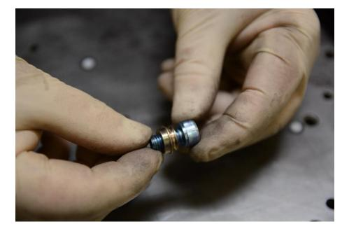
**Step 8**Apply blue Loctite to allen bolt
